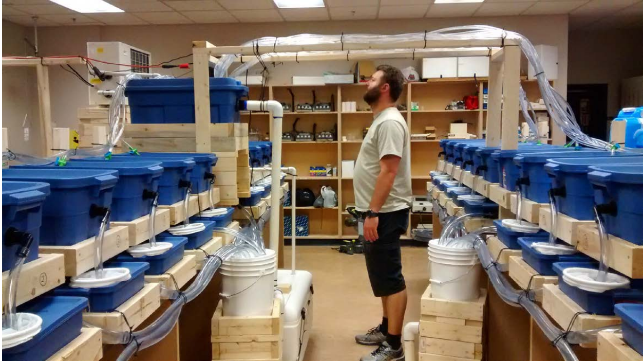
Figure 9 Overview of laboratory setup 3. The photo shows a partial overview of the laboratory setup. It shows the header tank (blue tank at upper left), fish holding tanks (larger), filter tanks (smaller), the two biological filters (two white buckets), the sump (white cooler at lower center), and chiller (white box at upper left, in the background), and the tubing connecting the various parts. Note the large overflow pipe returning excess water from the header to the sump. Also, note that the filters (white rings) were removed from the filter tanks, due to problems with clogging and flooding. (Photo: Melissa Mageroy)
