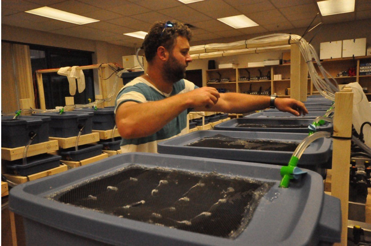
Figure 10 Fish holding tanks 1. The photo shows the screened lids of the holding tanks and the stop cocks regulating flow into the tanks. (Photo: Ian Walker)
