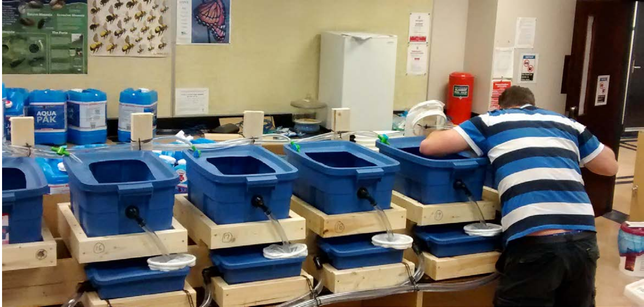
Figure 11 Fish holding tanks 2. The photo shows the fish holding tanks (larger) and filter tanks (smaller). Note that the filters (white rings) were removed from the filter tanks, due to problems with clogging and flooding. (Photo: Melissa Mageroy)
