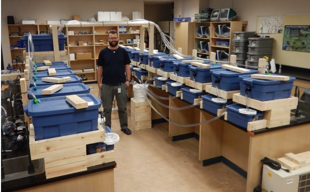
Figure 8 Overview of laboratory setup 2. The photo gives an overview of the laboratory setup during construction. It shows the header tank (upper left), fish holding tanks (larger) with filter tanks (smaller), one of the biological filters (white bucket), and the tubing connecting the various parts. At this point in time, the sump, chiller, and UV-filtration system was not installed. Note that the filters (white rings) were removed from the filter tanks, due to problems with clogging and flooding. (Photo: Ian Walker)
